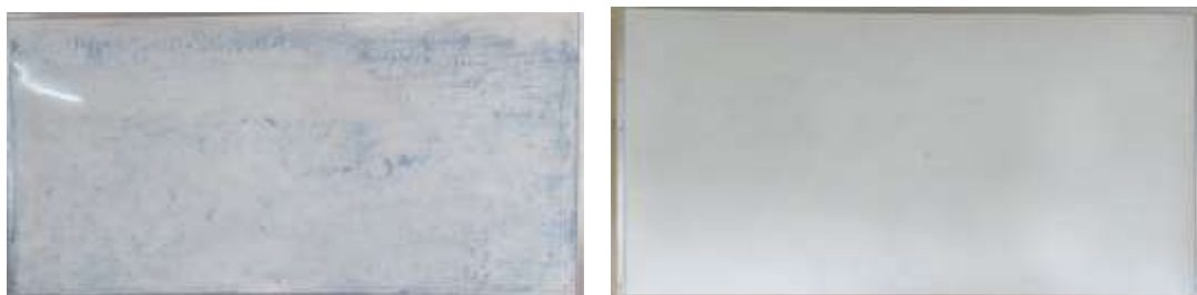
Figure 9. Before and after cleaning of whiteboard with 50% eco-enzyme
